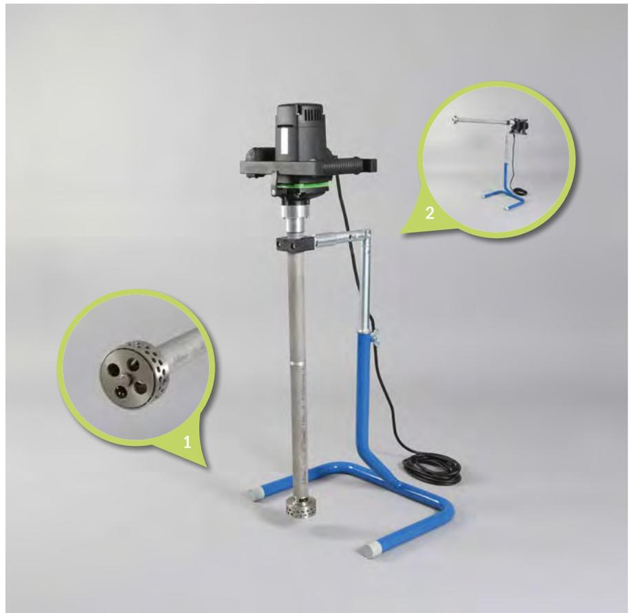
1. Rührkopf (Kolloidalmischer) | Mixing head (Colloidal mixer)
