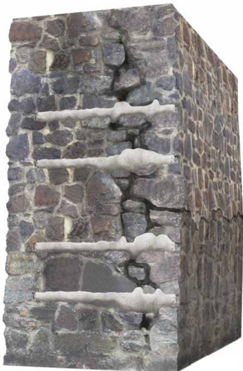
Fig. 4 Connection of separated wythes
